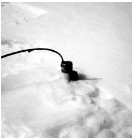
Figure 3. The placement of the thermometers in the snow.
