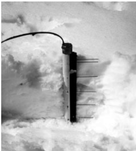
Figure 2. The thermometers used by the scientists.
