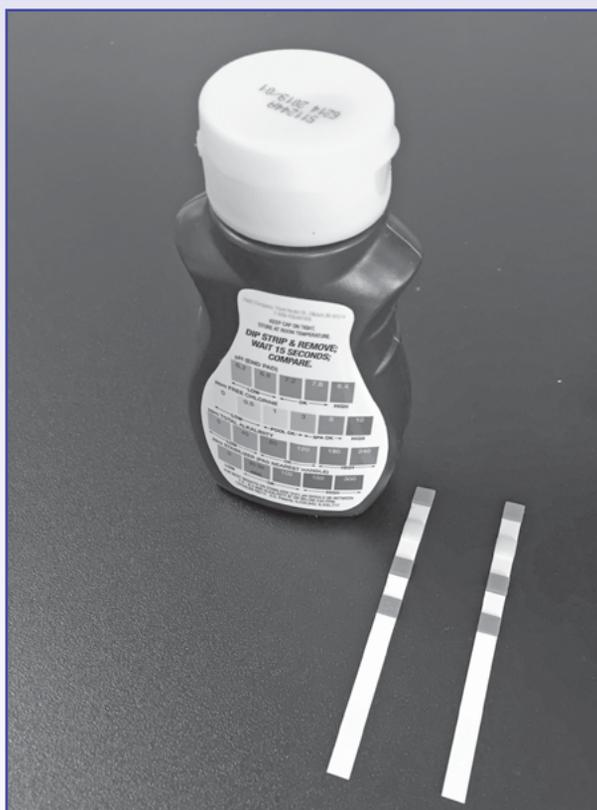
**Figure 14.** Compare the chlorine test strip pad color with the free chlorine color key on the back of the test strip bottle.
